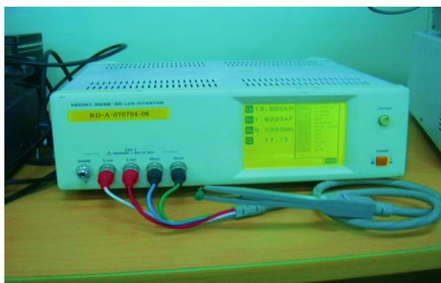
Figure (2): Conductivity measurements (Hioki, 3532-50 LCR Hitester).
