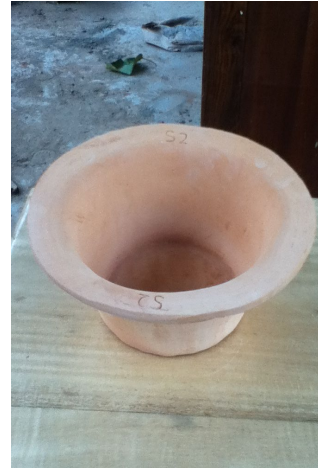
Plate 9: Fired filter sample
