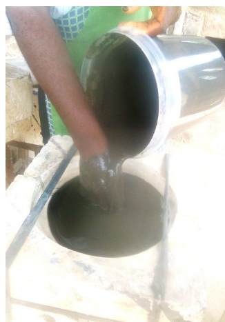
Plate 4: Slip-casting of filter samples
