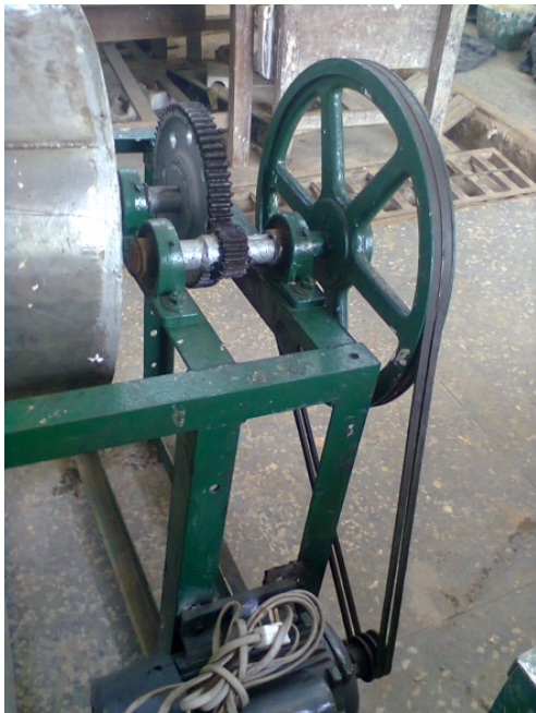
Plate 3: The Motion Transmission System Photo: Oresangun, A.O. fieldwork (2012)
