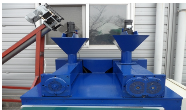
Figure1: Image of the experimental pelletizing instrument developed for this study
